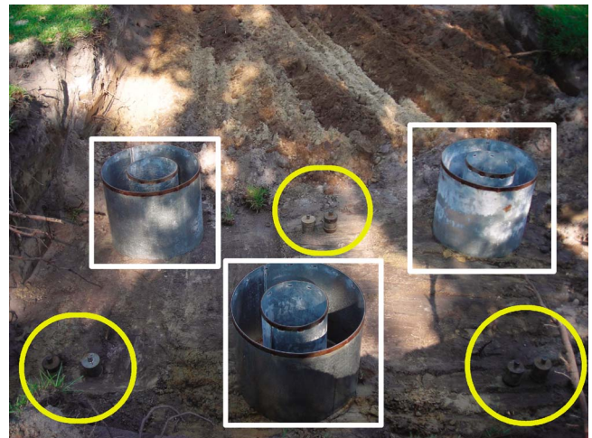
Fig. 3. Layout of soil cores (circles) and double-ring infiltrimeters (rectangles) in the field for the site that employed the scoop method. The soil texture from the rake method can be seen in the top of the photo.
