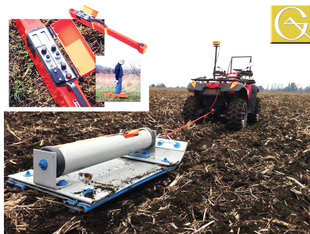
Fig. 6.12. EM-38 sensor, and electromagnetic sensor, courtesy of Geonics, Ltd., Mississauga, ON.
