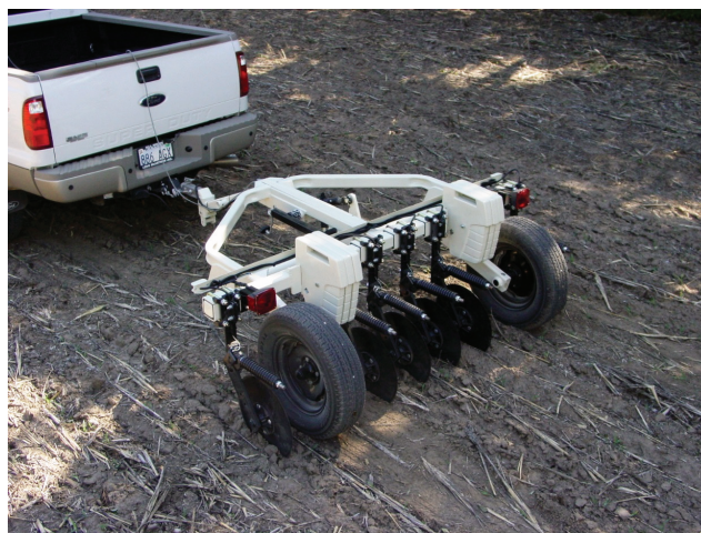
Fig. 6.11. Veris Technologies soil EC sensor. Courtesy of Veris Technologies, Salinas, KS.
