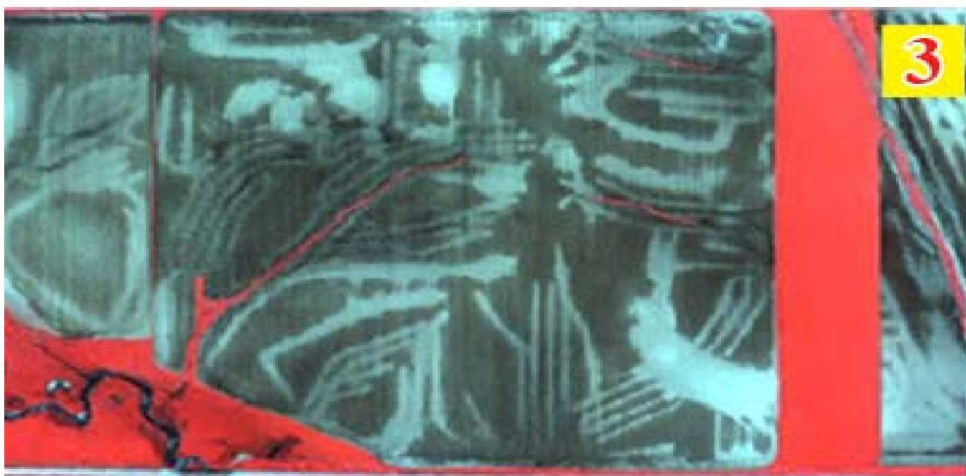
Image 3 is the same field shortly after a rain. Lighter areas are where soil is dryer. The parallel lines in this image show where tile drainage lines are located in the field.
