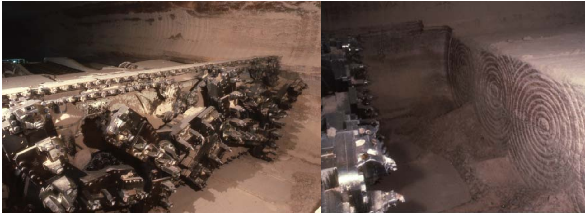
“Drum-type” continuous mining machine
