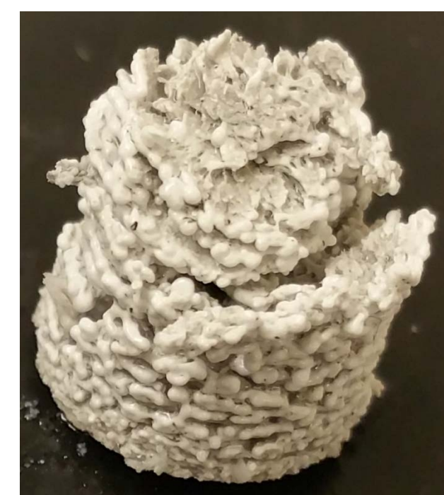
ZSM-5 remains after bomb calorimetry
