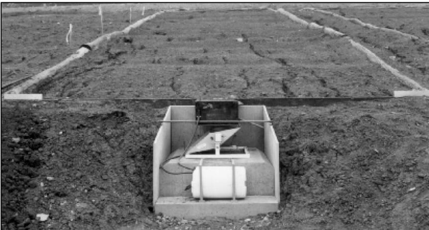
**Fig. 6-6. Photograph of a 20-m long by 5- m wide runoff plot in Queensland, Australia. This plot is equipped with a tipping bucket device to measure runoff. Reproduced from Carroll et al. (2000).**
