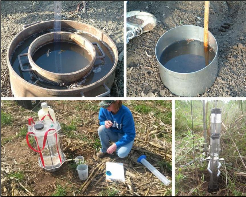
**Fig. 6-5.** Photographs of a double-ring infiltrometer (top left; Source: Wikipedia, public domain), single-ring infiltrometer (top right; Source: Wikipedia, public domain), mini-disk tension infiltrometer (bottom right), and sprinkle infiltrometer (bottom left, Source: Iowa Learning Farms, used by permission).
