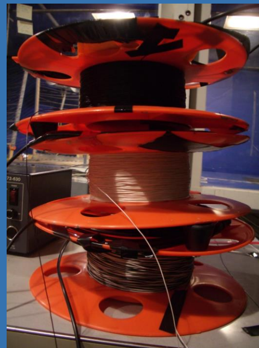
Fiber diameter 0.9 mm Black and white jackets
