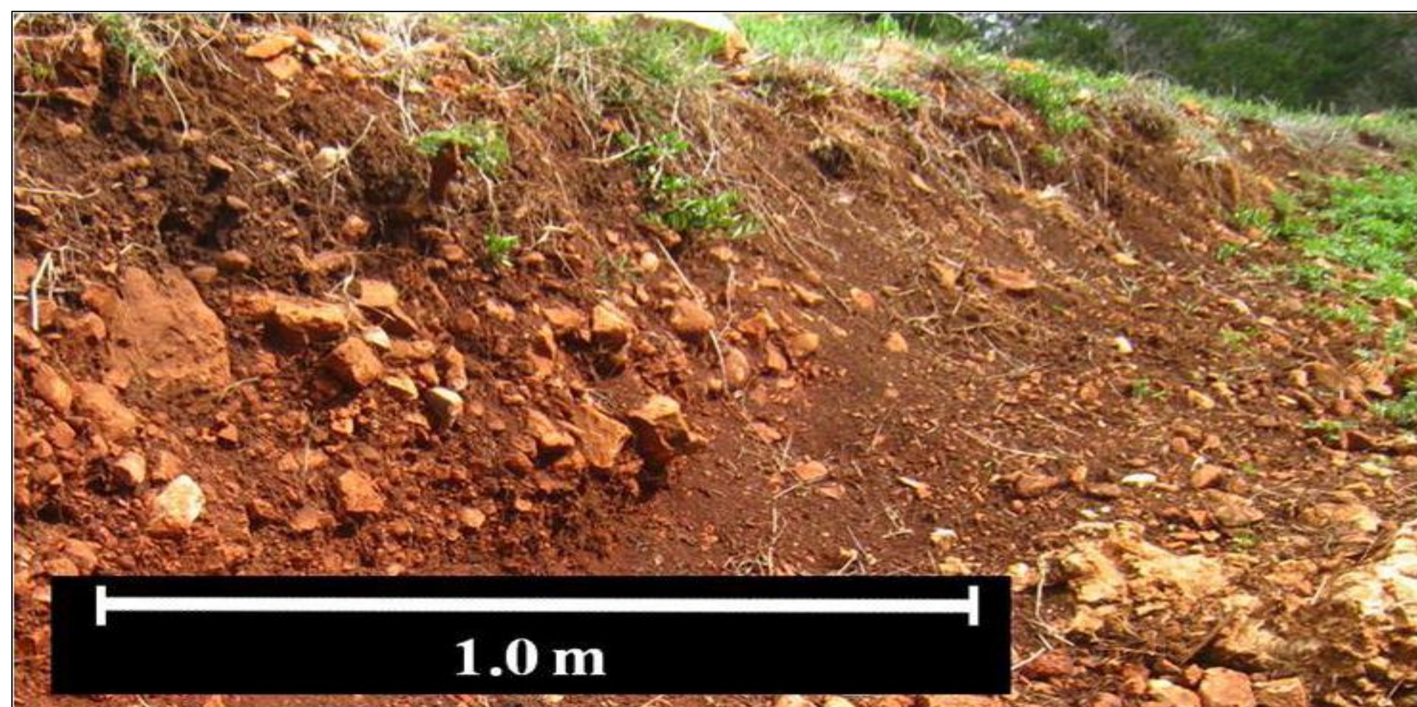
Fig. 1 Profile of the Rumble gravelly clay loam at the Freeman Ranch Center of Texas State University near San Marcos, Texas. Photo taken by Dr. Ieyasu Tokumoto.
