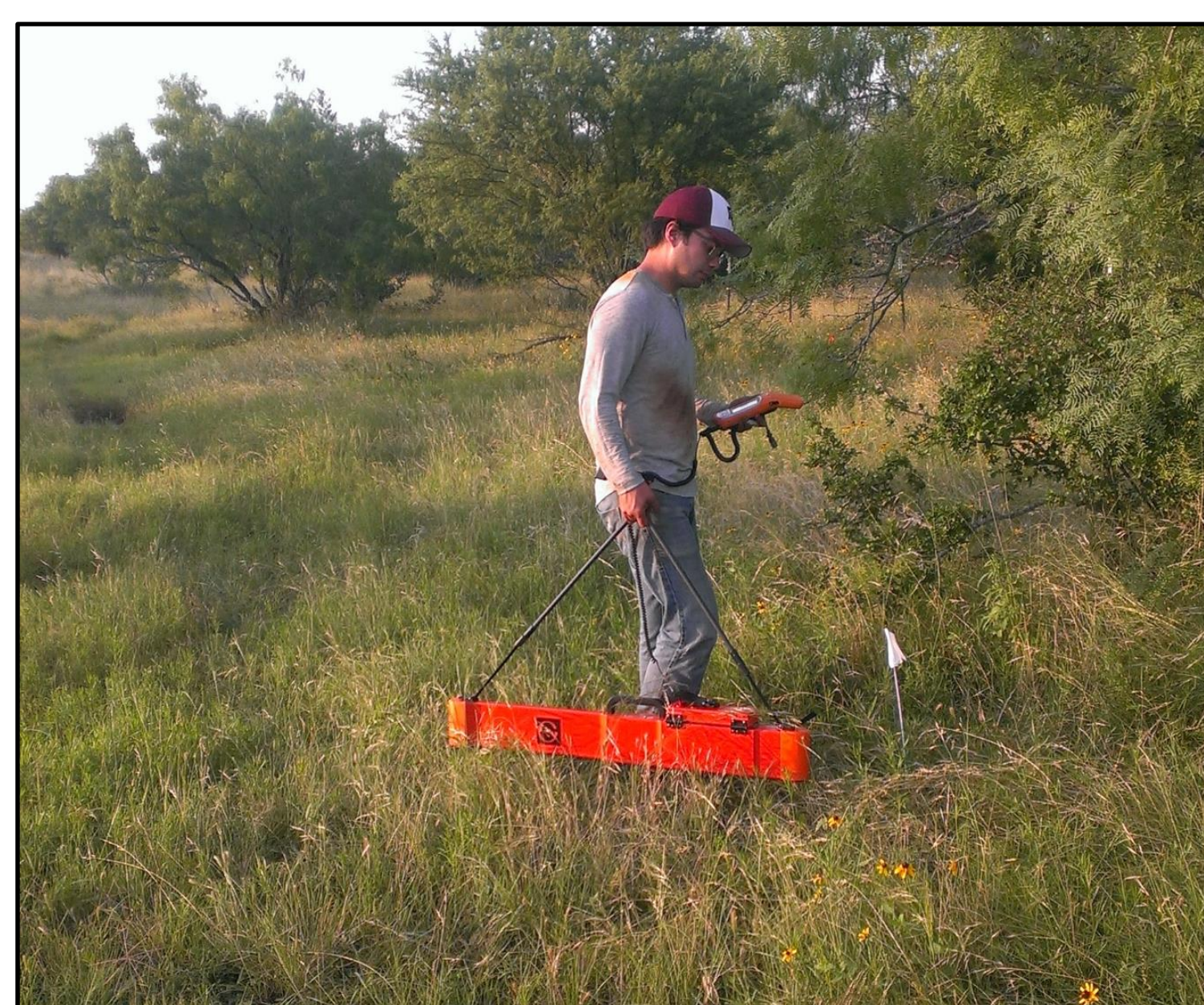
Fig. 2 Conducting an EMI survey.
