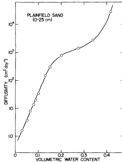
Fig. 3—Soil-water diffusivity as a function of volumetric water content for the 0-25-cm depth of Plainfield sand.
