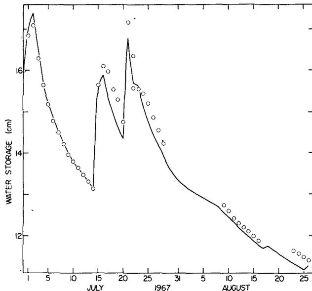
Fig. 8—Predicted soil water storage (solid line) in bare Plainfield sand compared with that measured by lysimeter (circles).
