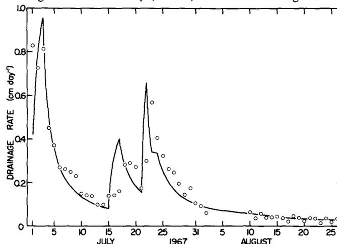
Fig. 7—Predicted drainage (solid line) from bare Plainfield sand compared with that measured by lysimeter (circles).
