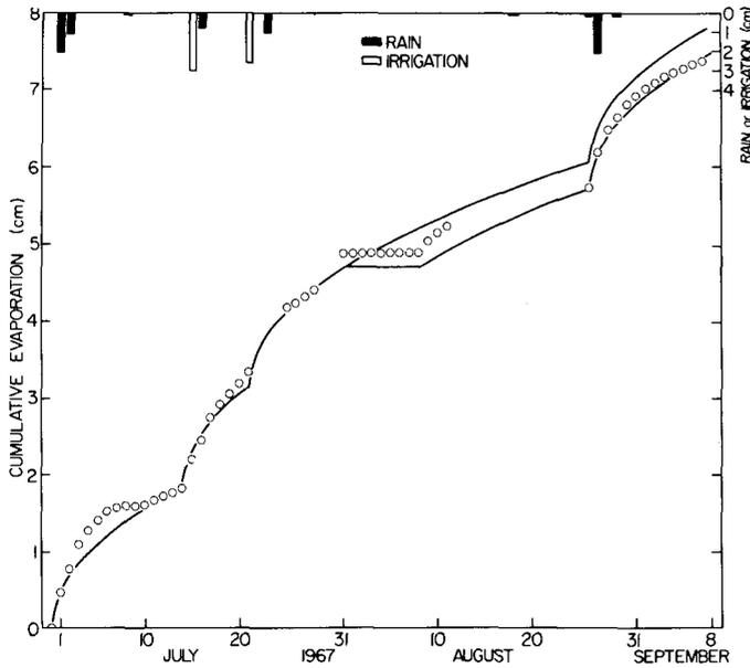
Fig. 5—Predicted cumulative evaporation from bare Plainfield sand compared with that measured by lysimeter. The circles are lysimeter data. The smooth curves were obtained using [6] with  $C = 0.496 \text{ cm day}^{-1/2}$  and setting  $t = 0$  after each heavy rain.
