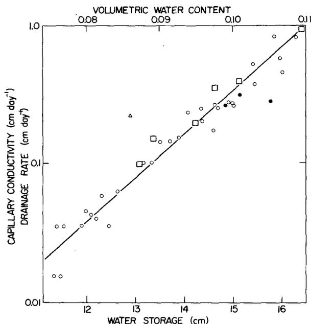
Fig. 6—Lysimeter drainage rate as a function of water storage (circles) and capillary conductivity of Plainfield sand as a function of soil water content (squares). The upper scale gives the soil water content corresponding to a given storage assuming a uniform water content distribution.
