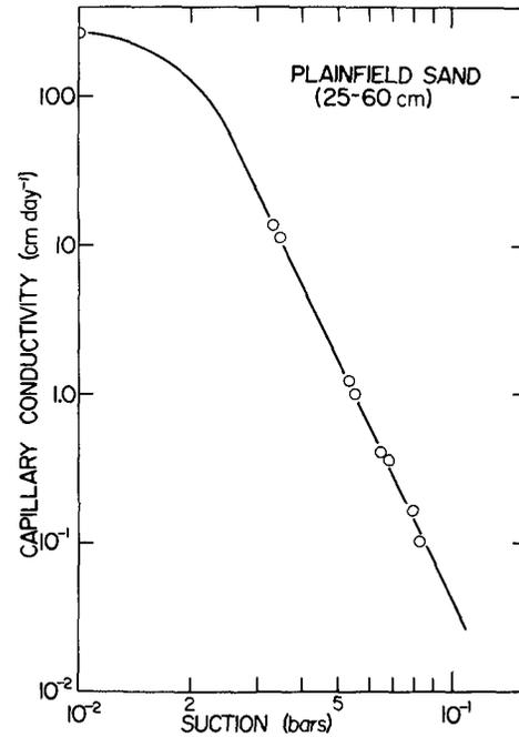
Fig. 2—Capillary conductivity as a function of soil-water suction for the 25-60-cm depth of Plainfield sand.
