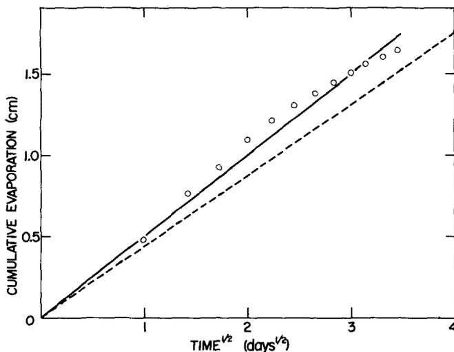
Fig. 4—Cumulative evaporation from bare Plainfield sand as a function of  $t^{1/2}$ . The circles are lysimeter data from Aug. 27 to Sept. 7, 1967. The solid line is the best fit by eye to the lysimeter data, while the dashed line is for  $\bar{D} = 10 \text{ cm}^2/\text{day}$  obtained from laboratory data.
