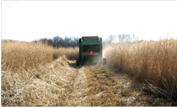
Figure 6-2. Harvesting switchgrass in a windrow with a round baler.
