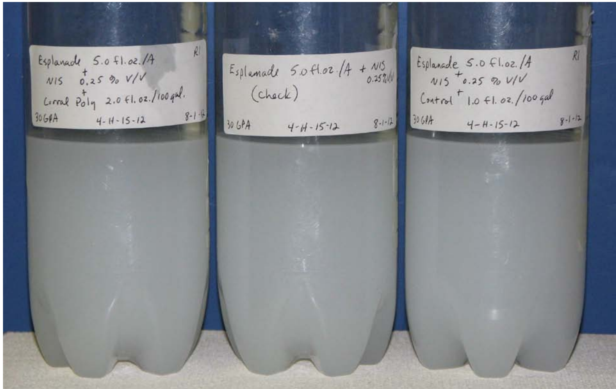
Figure 1. Compatible mixture of Esplanade™ 200 SC and Corral® Poly (bottle on far left) and Control™ mixture in the far right bottle. Bottle in the middle is a controlled check with only Esplanade® 200 SC and non-ionic surfactant.
