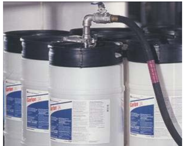
Figure 4. Micro Matic valve and couple attached to bulk container.
