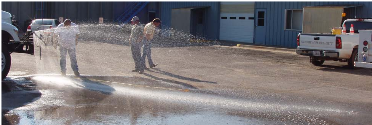
Figure 3. Boominator® 5000R spray tip mounted at a height of 48 inches and operating at 25 psi.
